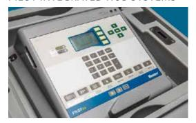
Integrated hub systems are one of the fastest-growing forms of technology in irrigation control. A key advantage over field controller systems is that integrated hub systems use significantly less wire. This means lower costs, faster installation, and easier system diagnosis and repair if needed. Systems can be easily expanded — with minimal digging and disruption of landscaping - by adding more two-way modules (TWMs) instead of running additional wires.
