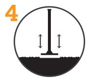
Work moisture into clay and compact until firm with tamp. Cover mound clay with conditoner or infield mix.
